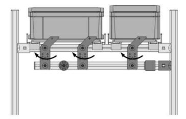
The Release Unit can perform the same function even on protruding roller conveyors.
